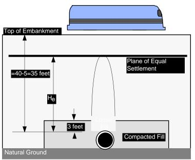
To avoid deformations at the surface of the conduit means than the design must result in a "plane of equal settlement" below the surface of the embankment.
