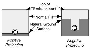
lines. There are two variations: the Positive Projecting and the Negative Projecting conduit, shown to the right.
