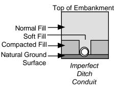
prism above the conduit, making in effect a negatively projecting conduit.
